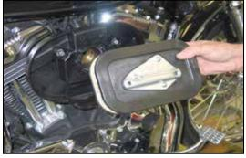
4. Remove the air filter as shown.
