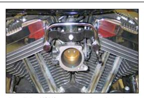
7. Install the K&N® crankcase breather tube onto the vehicle using the provided hardware. NOTE: Do not completely tighten the breather bolts at this time.
