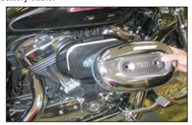
2. Remove the two air filter cover mounting bolts and then remove the cover from the vehicle as shown.
