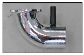
9. Cut the provided crankcase vent hose to a length of 1.75" and install onto the  $K\&N^{\otimes}$  intake tube as shown.
